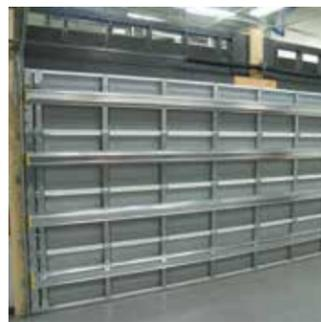
Raynor Hurricane Ready reinforcing systems utilize horizontal trussing, made from high-tensile steel box struts or u-bars, to create a door system built to withstand hurricane force winds.
